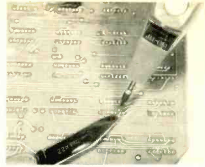
FIG. 6—PINS AND LEADS must be straightened before components can be removed.
