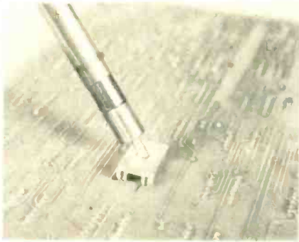
FIG. 8—DIP DESOLDERING TIP heats all pins at the same time
