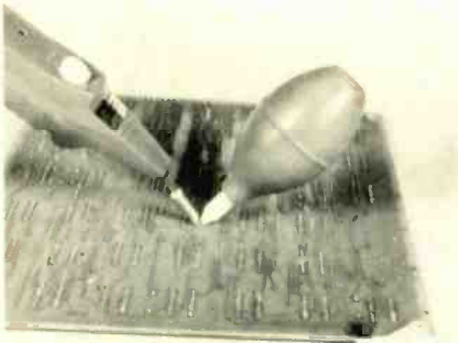
FIG. 3—SEPARATE VACUUM BULB and solder iron is not as effective as combination unit since each tip must make room for the other. Also, two hands are required for this method.
