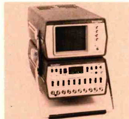
MULTITRACE SCOPE by Gould aids analysis in complex digital pulse stages and circuits, but dual-trace model suffices for VCR diagnosis.
