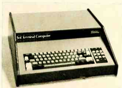
SOL TERMINAL COMPUTER has computer and alphanumeric keyboard in a single enclosure.
