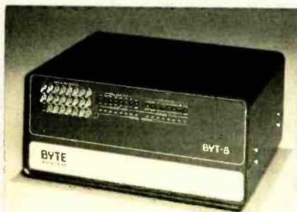
BYT-8 microcomputer from Byte Incorporated has toggle switches and LED indicators on the front panel.
