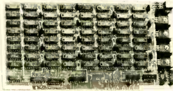
STATIC RAM MEMORY from Vector Graphic is designed for the S100 bus structure.
