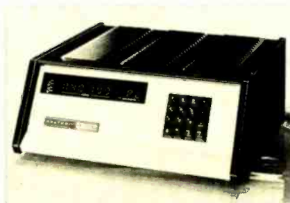
HEATH H8 computer has an octal display and keyboard on the front panel.
