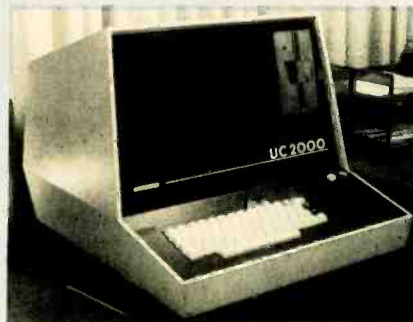
UC-2000 from Infinite Systems contains computer, CRT terminal, and floppy disc drives.
