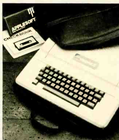
CONNECT A TV SET to the Apple II computer and you have a computer and CRT terminal.
