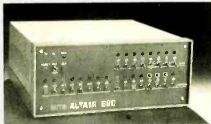
ALTAIR 680 FROM MITS has toggle switches and discrete LED indicators on front panel.
