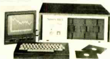
SYSTEM 8813 from Polymorphic has three floppy disk drives.
