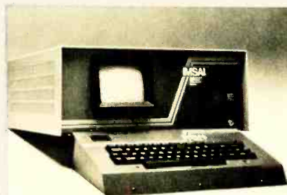
IBK-1 MICROCOMPUTER from IMSAI has built-in card cage, CRT terminal and power supply
