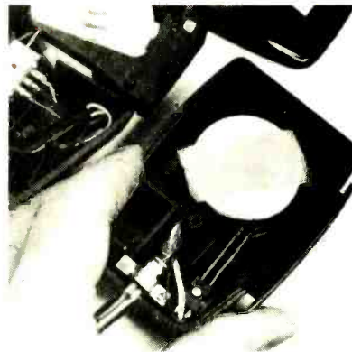
SOME MICROPHONES USE A LEAF switch (right), while others use a plunger-type DPDT switch.
