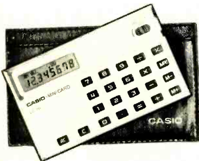
CASIO LC-78 MINI-CARD CALCULATOR is no bigger than a credit card, yet offers four math functions, percent and memory.
