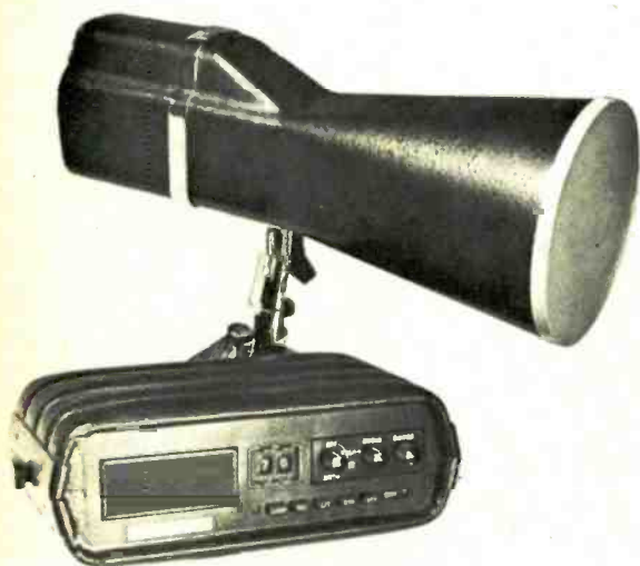
TYPICAL POLICE RADAR UNIT. The antenna can be remotely positioned when necessary. It reads out directly in MPH.
