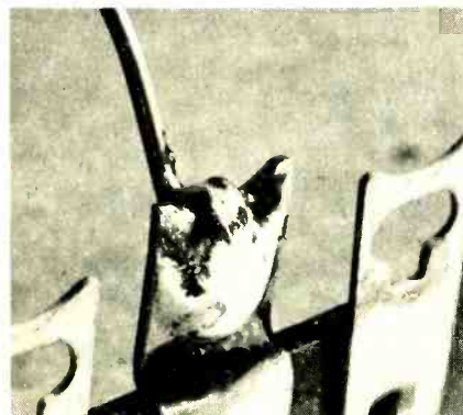
SOLDERED JOINTS, GOOD AND BAD, depend on tools, solder, temperature and technique. Left photo shows the dull solder surface of a poor joint. Good joint (right) has a bright silvery surface.
