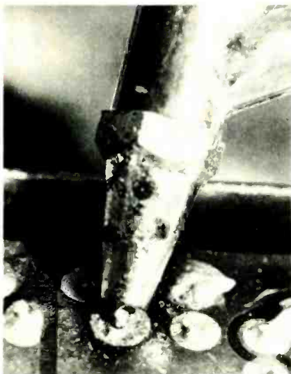
THIS SOLDER JOINT HAS just been desoldered. The hot solder has been sucked away leaving a component pin that will easily pull free from the circuit board.
