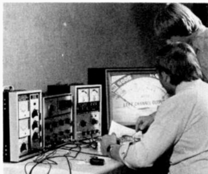
A HIGHLIGHT OF THE RECENT SENCORE troubleshooting seminar was the company's all-in-one AM/FM/stereo and CB analyzer, developed to help service in-dash combo units.
