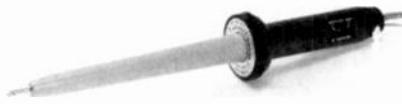
FIG. 4—TO MEASURE really high voltages—such as the 30-kV boost voltage often found in a color TV—some form of attenuator is essential. This special probe provides 100-times attenuation using highly accurate resistors. The length of the probe provides some protection for the user.
