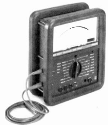
FIG. 9—EVEN THE BEST cared for service instrument sometimes slips, or is knocked against a tool. Some sort of protection—such as the rubber rings mounted on this meter—are useful.
