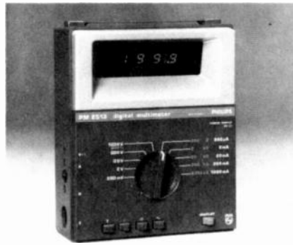
FIG. 6—CHOOSING BETWEEN ANALOG AND DIGITAL INSTRUMENTS often has to be a matter of personal choice. A digital meter is better for accurate measurements, while an analog meter is ideal for peak-and-dip and other trend readings.
