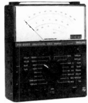
FIG. 6—CHOOSING BETWEEN ANALOG AND DIGITAL INSTRUMENTS often has to be a matter of personal choice. A digital meter is better for accurate measurements, while an analog meter is ideal for peak-and-dip and other trend readings.
