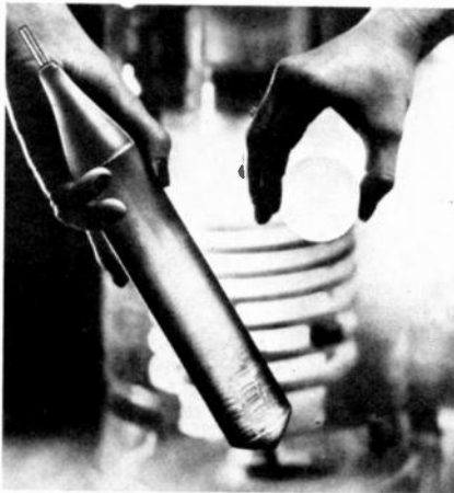
GADOLINIUM GALLIUM GARNET single-crystal boule and wafer.
