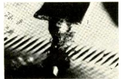
FIG. 3—MICROPHOTOGRAPH OF STYLUS tracing groove of untreated record.
