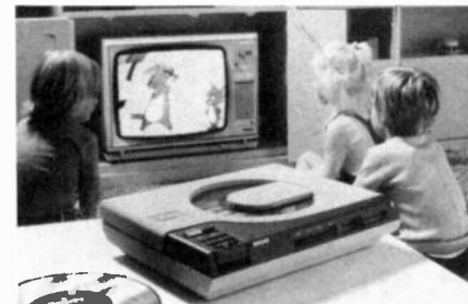
VIDEOPLAYER developed by Philips to play its VLP (Video Long Play) discs. Signal is fed to set's antenna terminals.
