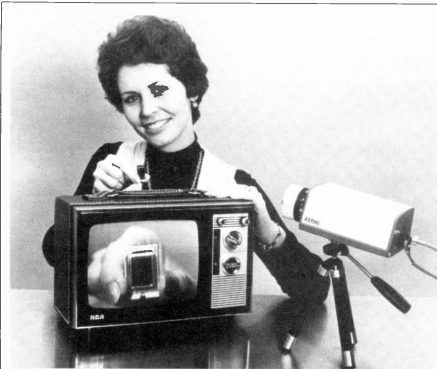
THE CHARGE-COUPLED IMAGE SENSOR of the new solid-state television camera is the largest and highest resolution device of its kind yet made. Production in sample quantities is scheduled for the second quarter of 1975.
