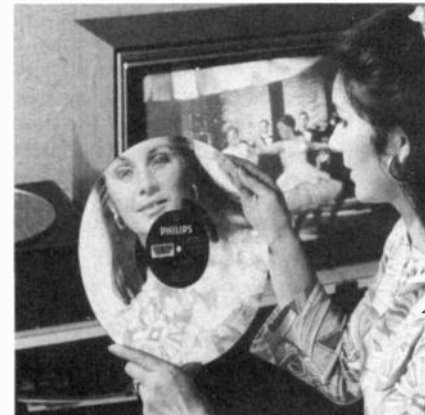
VLP DISCS ARE TRANSPARENT RIGID PLASTIC with a thin reflective metal layer. Duplication is by stamping from glass master.
