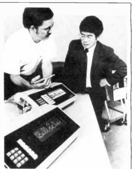
FLAT PLASMA SCREEN VIDEO DEVICE demonstrated by developers Eugene Sampiere and Peter Ngo, can not only transmit handwriting, but other forms of graphic display, and enables the user to "talk to the computer."
