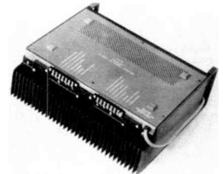
MASSIVE HEAT SINKS cover the entire rear panel of the power supply.
