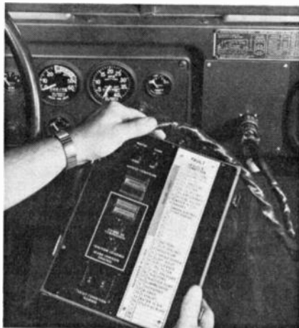
AUTOMOTIVE VEHICLE TEST SYSTEM, built by RCA, can reduce checking time by 90%.
