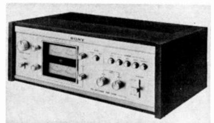
FIG. 5—WAVE COMPARATOR used in this and other expensive decoders has front-to-back and side-to-side logic circuitry.
