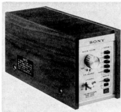
FIG. 3—SONY SQD-2050 DECODER features logic circuits to enhance the otherwise poor front-to-back separation of the SQ system.
