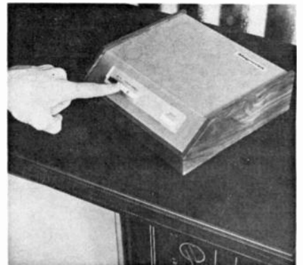
HOME TERMINAL CONTAINS CHANNEL switches and an "accept" button. Pushing either premium channel switch gives a preview of its program. The third switch is for ordinary CATV.
