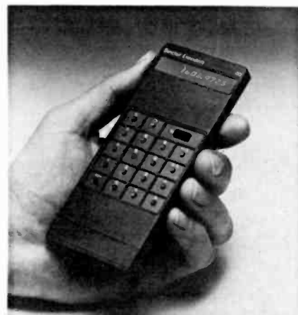
HAND-HELD ELECTRONIC CALCULATOR only \frac{3}{8} inch thick contains 7,000 transistors.
