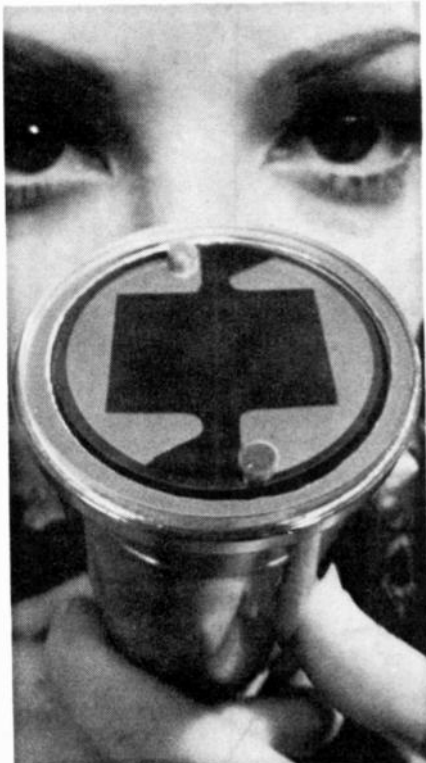
BIVICON CAMERA TUBE has two distinct pick-up surfaces—the dark rectangular area.
