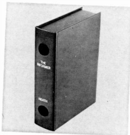
ULTRASONIC INTRUSION SENSOR by Heath-kit looks just like a book.
