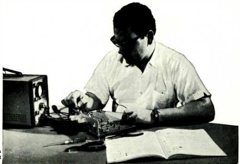
Performing transistor experiments on programmed breadboard—using oscilloscope.
