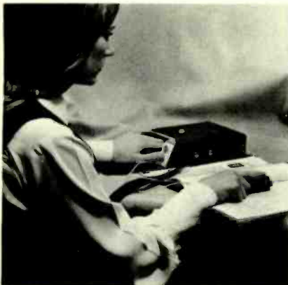
THE OPTACON used by the blind to read conventional print.
