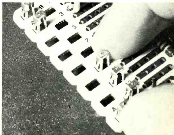
FIG. 11—CLOSE-UP OF DURA-MODULE contact (below). Notice that rows are numbered across the end.
