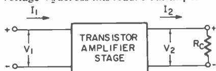
FIG. 1—HYBRID PARAMETERS are developed with this circuit. R_C is collector resistor in the transistor circuit.
