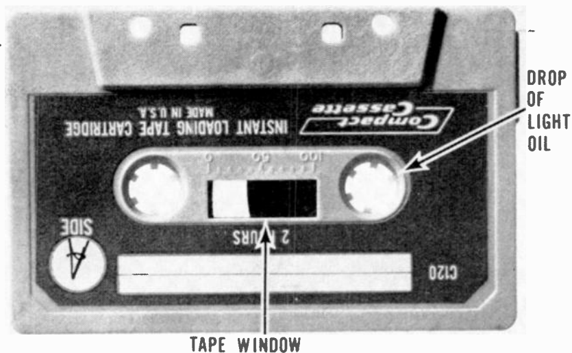
FIG. 2—A DROP OF LIGHT OIL at the hubs of tape cassette can prevent tape slowdown. Don't let any oil get onto tape itself.
