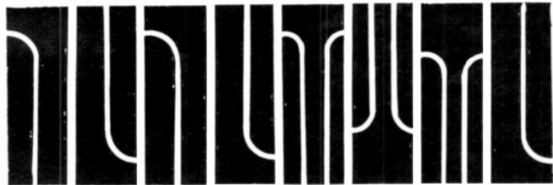
COMPONENT MOUNTING STRIP. Each strip contains 3 sections for diodes, capacitors or resistors, 1 transistor section and 1 SCR section.
