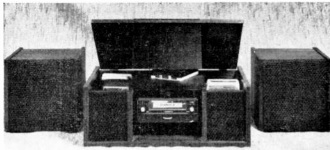
FOUR-CHANNEL TAPE PLAYER FOR THE HOME is made by Gibbs Special Products Corp. Special quadrasonic matrix system converts this standard system to 4-channel playback.
