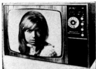
DIAL-A-PROGRAM being installed at Cape Cod, Mass. uses special color TV or conventional sets with converters. A multi-pair cable carries a 5-MHz to 10-MHz "super video" band of vhf/uhf signals.
