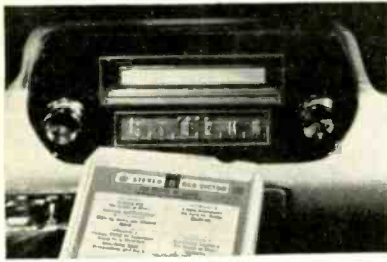
RCA Stereo 8 cartridge plugs into player in a modern car. Four 2-channel stereo program tracks are provided.
