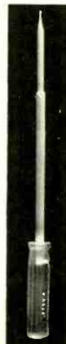
Fig. 1-b—Add a handle and you get a lot of added torque. Also helps to fine tune a coil. Shown is GC W2522.
