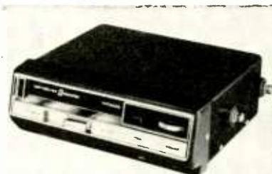
Hitachi CS-204 has dustproof door to protect player mechanism when not in use.
