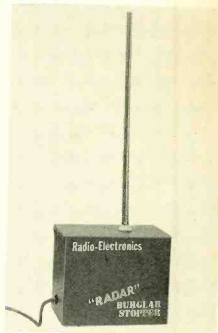
Build complete protection into your home or shop with R-E's tamper-proof, battery-powered burglar alarm
