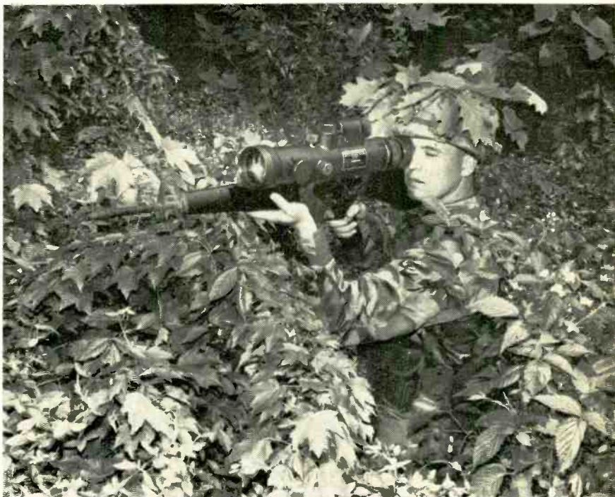
Rifle-mounted Starlight Scope has a 3" objective lens and 1/4-mile effective range.
