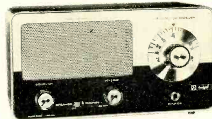
Fig. 6—Allied's Knight KG-220 is a vhf monitor in kit form. Two models cover low and high bands. Continuous tuning.
