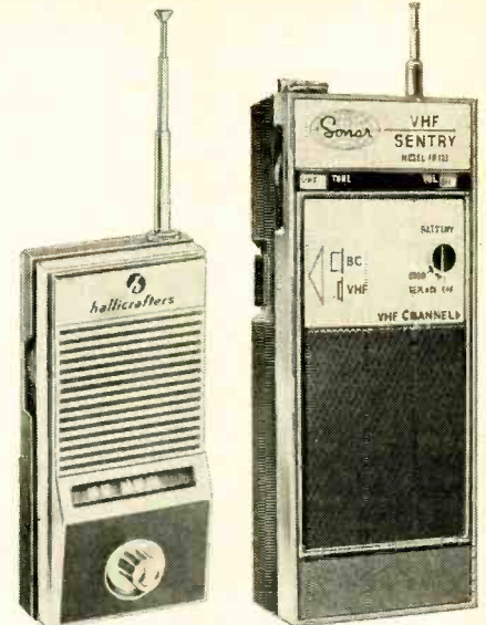
Fig. 12—Hallicrafters Portamon series also covers three major vhf bands and is portable. Has continuous tuning. $40.
