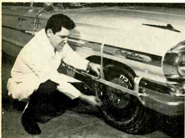
Fig. 3—For road testing, a loop antenna is installed near the wheel-mounted transmitter. Strip chart records signals.
