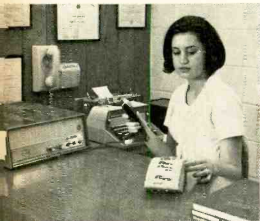
Fig. 10—Two-way FM base stations are often self-contained, like this RCA model.
