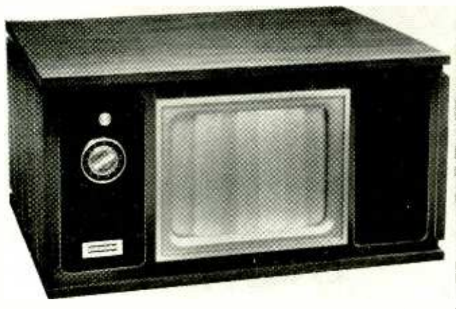
Experimental color set designed by Fairchild for Paramount Pictures C6003 Chromatron. This is the set described in this story.
