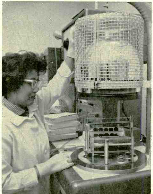
Evaporation apparatus like this is used for depositing interconnects.
