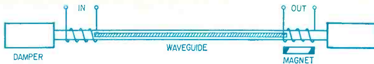
Fig. 5—Simplest magnetostrictive delay line.
