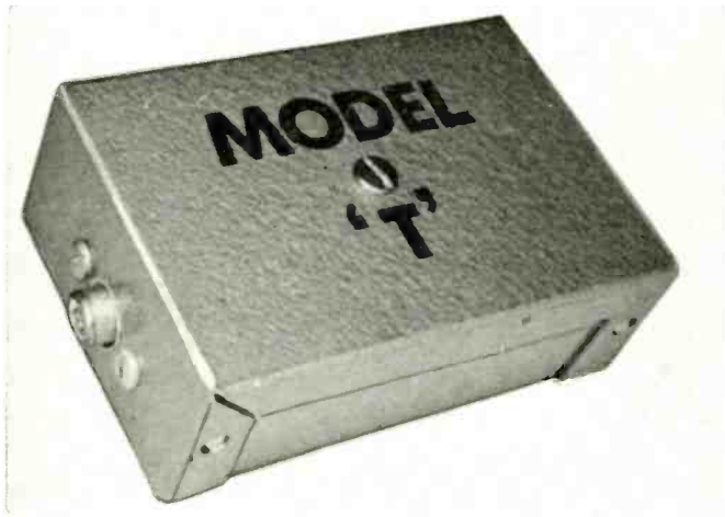
A single parallel-T filter for 19 kc.
