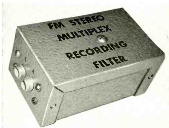
Dual parallel-T's for stereo (38 kc).
