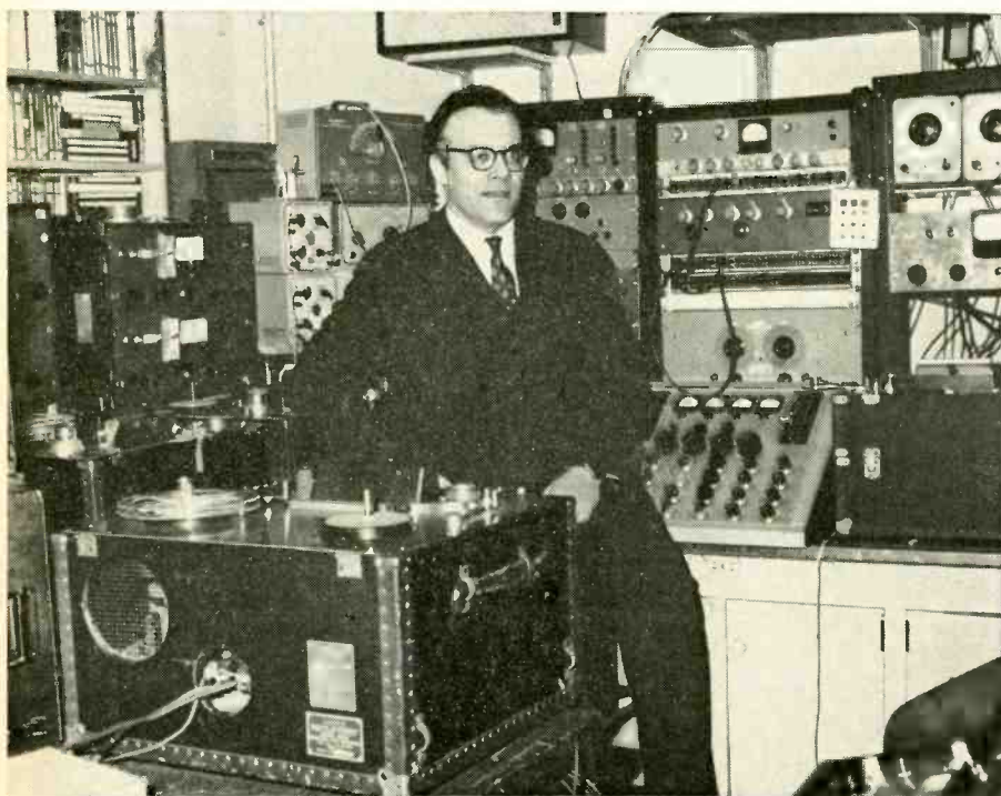
Vladimir Ussachevsky, Chairman of the Committee of Direction of the Columbia-Princeton Electronic Music Center, in the older studio of the Center, which still contains some of the original equipment with which he and Otto Luening began to work in 1952. To Ussachevsky's right are tape recorders, electronic switches, and sine- and square-wave oscillators. To his left are mixing, patching and filtering facilities and other tape recorders and oscillators.
