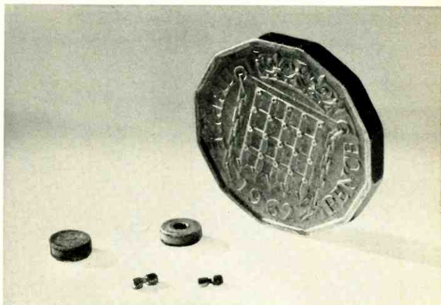
Two gallium arsenide lamps (rear) and two small semiconductor lasers. In the background, a British threepenny piece (slightly larger than a US cent) for size comparison.
