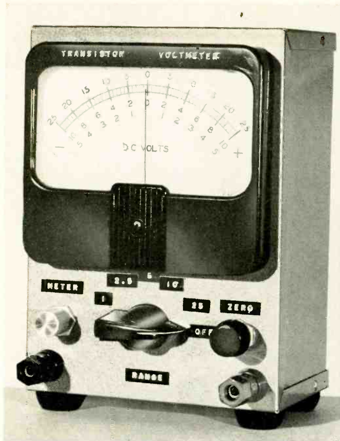
Zero-center meter eliminates need for interchanging probes or switching polarity. Neither input terminal is grounded to case.
