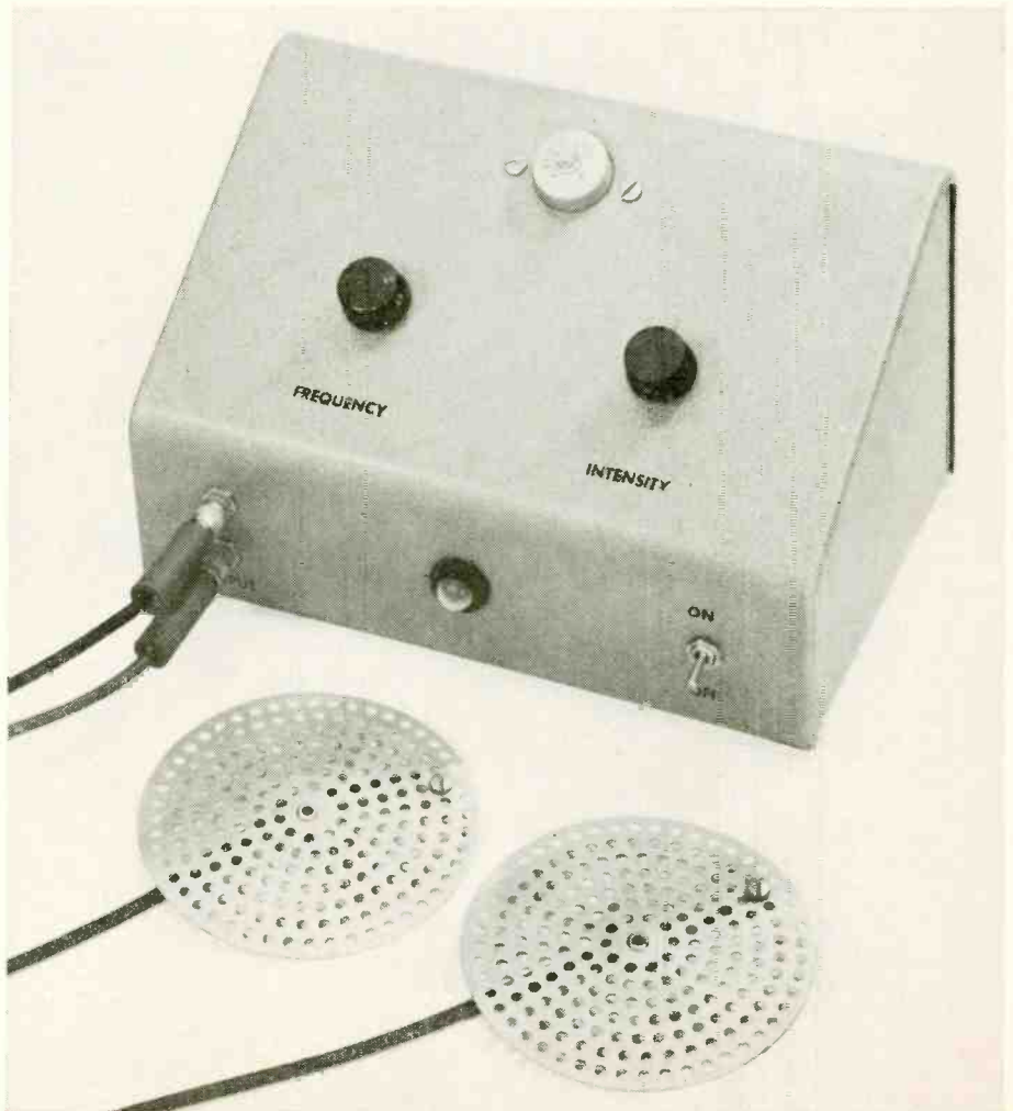
The complete Stimulator with its sink-drain electrodes in the foreground.
