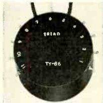
POWER SUPPLY TRANSFORMERS, TY-86 , are epoxy-molded toroidal, work from a 12-volt source and put out 350 dc ma at 425 dc volts. Designed for converting dynamotor supplies in transmitters to solid state power.—Triad Distributor Div., 305 N. Briant St., Huntington, Ind.
