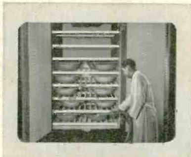
Drying ovens remove moisture from phosphor
