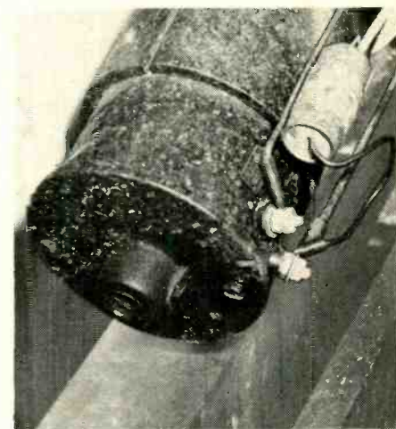
Fig. 3—Circuitry of Sonar D-60 is powered by internal battery inside housing. Boat's batteries operate motor.
