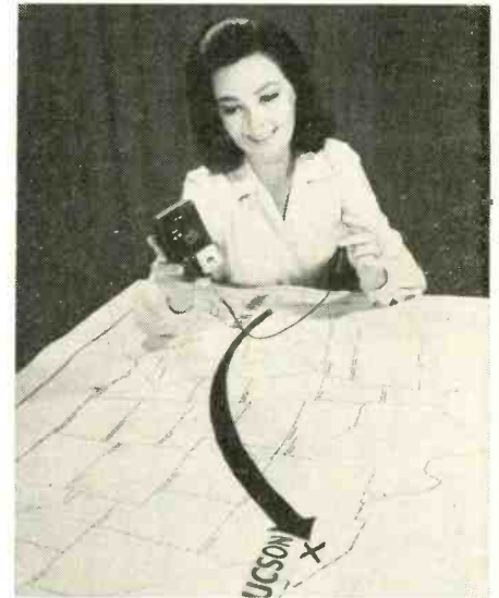
Crystal case (model's left hand) goes in armpit to keep temperature and frequency constant.
