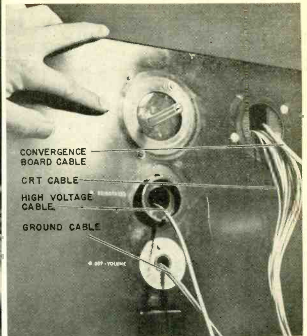
Photo 4—Extension cables protrude from control holes in mockup set. Bushings and dial plates from junkbox keep insulation from chafing on edges of holes. Plastic peg nearest hand is convenient for holding cables when mockup is not used.
