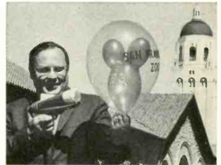
Stanford Prof. Arthur L. Schawlow demonstrates the principle of the laser eraser with his low-energy laser toy gun, which will burst the dark inside balloon, but not the clear outside one.
