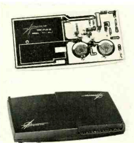
Top and interior views of the Multitron FM Stereo antenna. Antenna elements are the printed-circuit loops at the left in the interior photo.
