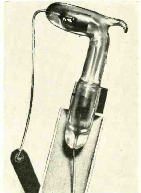
Fig. 2—Special neon bulb in Bendix DI-5 depth sounder.
