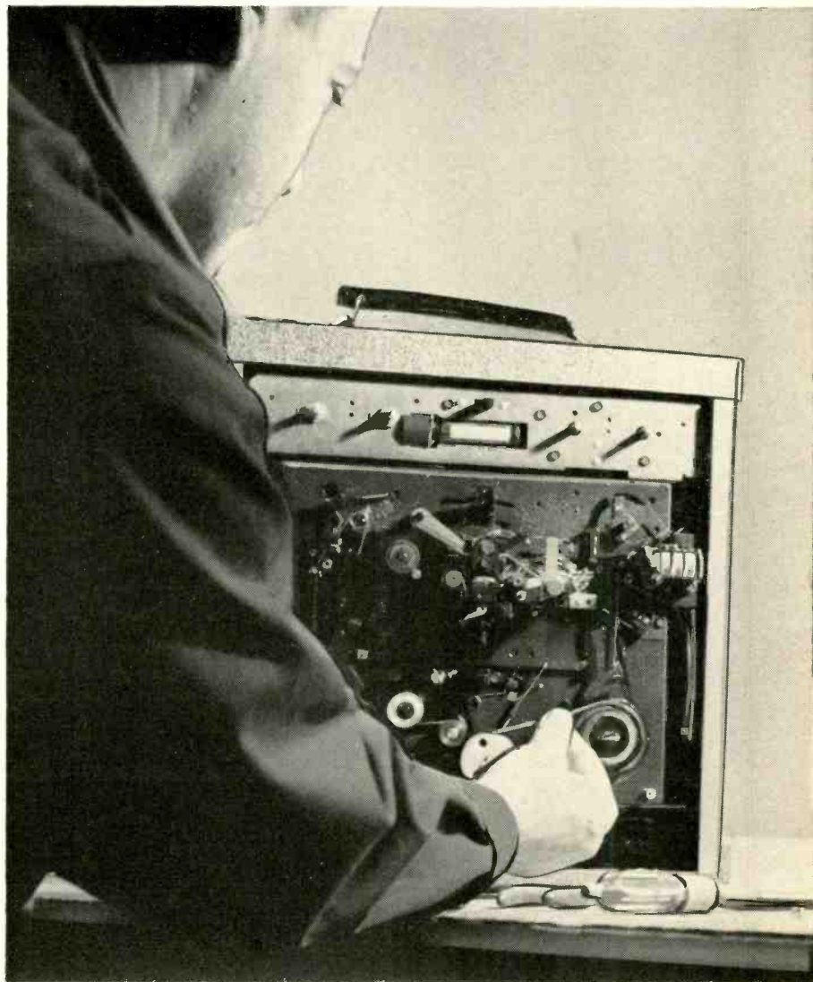
Art Margolis installs a new drive belt on a tape recorder.
