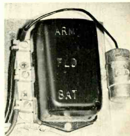
Fig. 4—Three standard spots to install noise suppression: coil (top), generator (center) and regulator (bottom).
