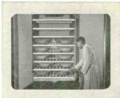
Drying ovens remove moisture from phosphor
