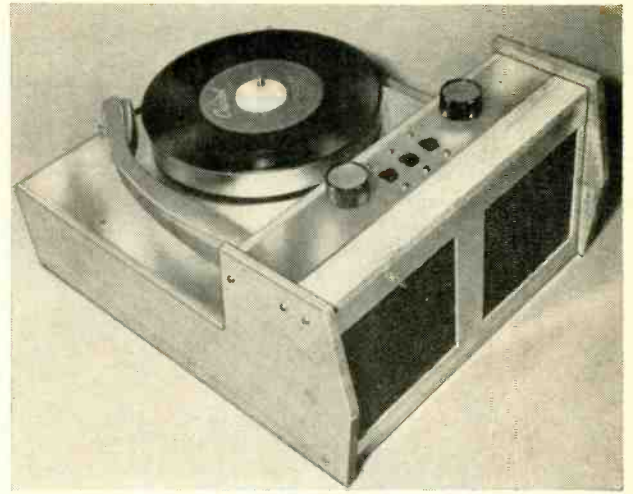
Two views of a miniature stereo phonograph using two amplifiers like ones described.
