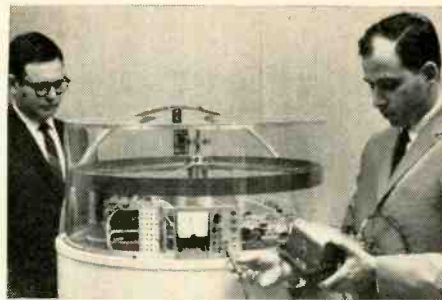
Project Director, Harold Perkel (left) and Dr. Robert Scher checking out a laboratory model of "Stabilite," the device that controls rocking, turning and twisting motions of an orbiting spacecraft.
