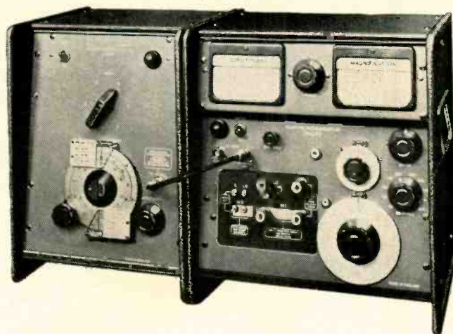
Marconi TF1245 Q meter connected to separate oscillator (left).
