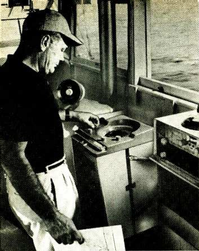
This radar, a Raytheon 1700, has a range of 12 miles. Targets are presented on 7-inch CRT.
