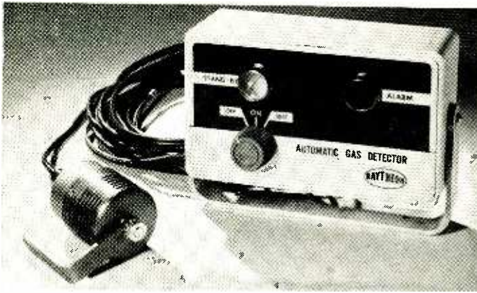
Gas detectors like this one use sensing unit (at left) and control unit, which carries warning light. Alarm light flashes when gas-fume accumulations in bilges or engine spaces reaches dangerous proportions.
