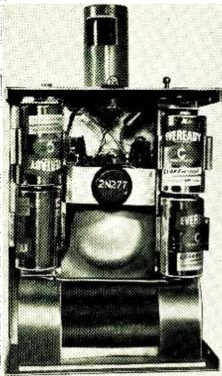
Symmetrically mounted batteries balance the weight of the slave flash unit.
