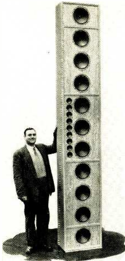
Wireless World Fig. 4—One of two 11-foot tall Pamphonic systems built in 1952 and used in the dome of St. Paul's Cathedral in London. There are eleven 10-inch and nine 3½-inch speakers, with crossover at 1,000 cycles. Frequency range is deliberately restricted to 250-4,000 cycles for best intelligibility.
