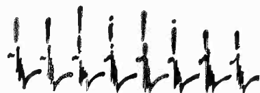
Fig. 3—Normal parade display shows all cylinders in a row.
