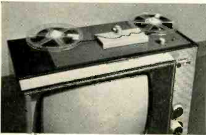
The video tape recorder measures 17 1/2 x 9 x 6 inches and weighs 15 pounds. (Below) Recorder built in as part of a TV receiver.
