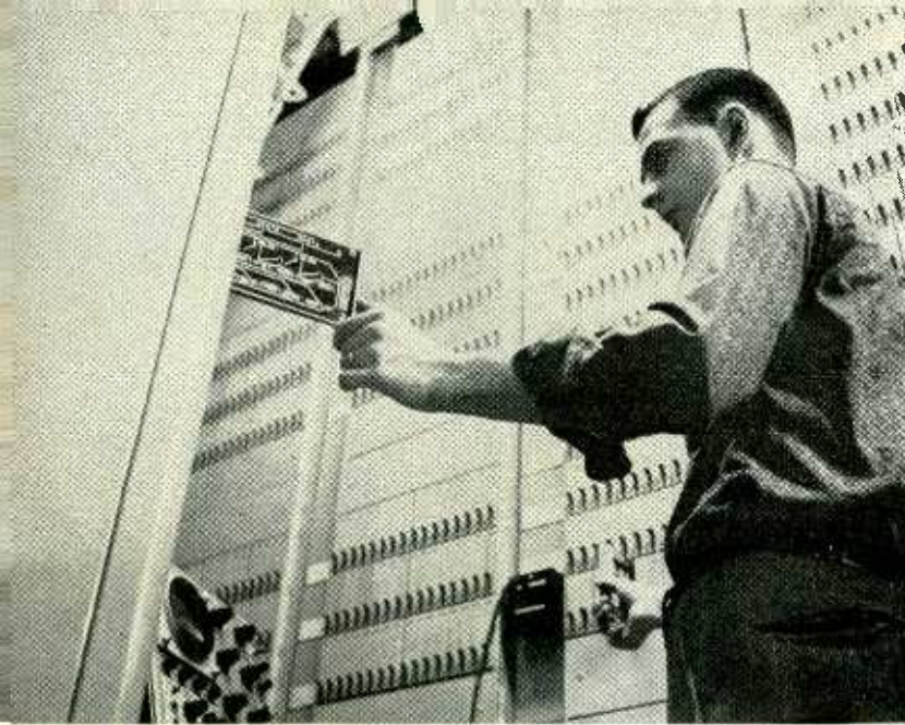
TASI terminal equipment uses 2,500 printed circuit cards.
