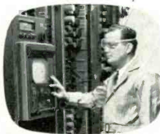
Precision Signal Generator sends out the test pattern shown on the screen above. Fidelity of reproduction of this virtual perfect signal (resolution: up to 2,300 lines!) is an accurate index of the picture tube's performance after life testing.
