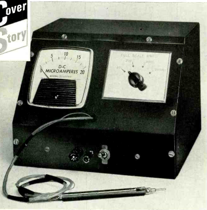
The meter. Binding post between fuseholder and switch is for ground lead, connected to one side of capacitor under test.
