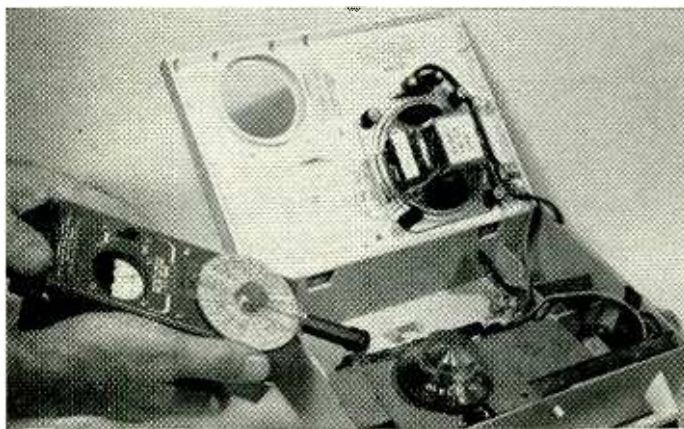
Using PACO G-15 to check ferrite antenna in portable radio.
