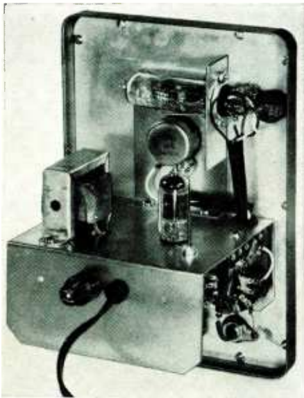
The in-circuit capacitance checker with its case removed.
