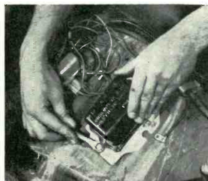
Install regulator in the same location as original regulator and wire it according to proper wiring diagram.
