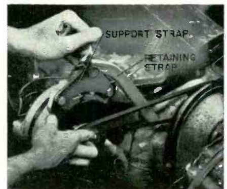
Adjust alternator position to allow for hood and fender clearances. Engage bolt to connect support strap to retaining strap.
