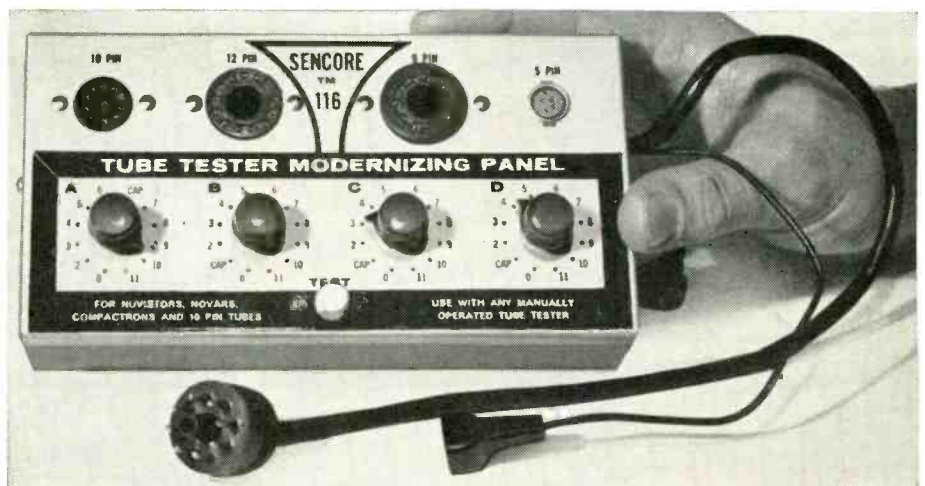
Sencore TM-116 plugs into octal socket on tube tester.
