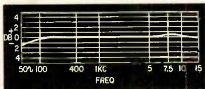
Fig. 2—Curve shows excellent frequency response of the portable, low-cost amplifier.
