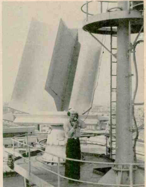
3-D RADAR ANTENNA on the masthead of missile cruiser USS Galveston simultaneously detects range, bearing and attitude of aircraft. Single antenna replaces two or more previously required to do the same job. Unit is part of Hughes Aircraft Frescan radar system.
