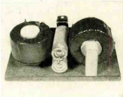
Two views of the completed crossover. Note the electrolytics nestled between the coils.
