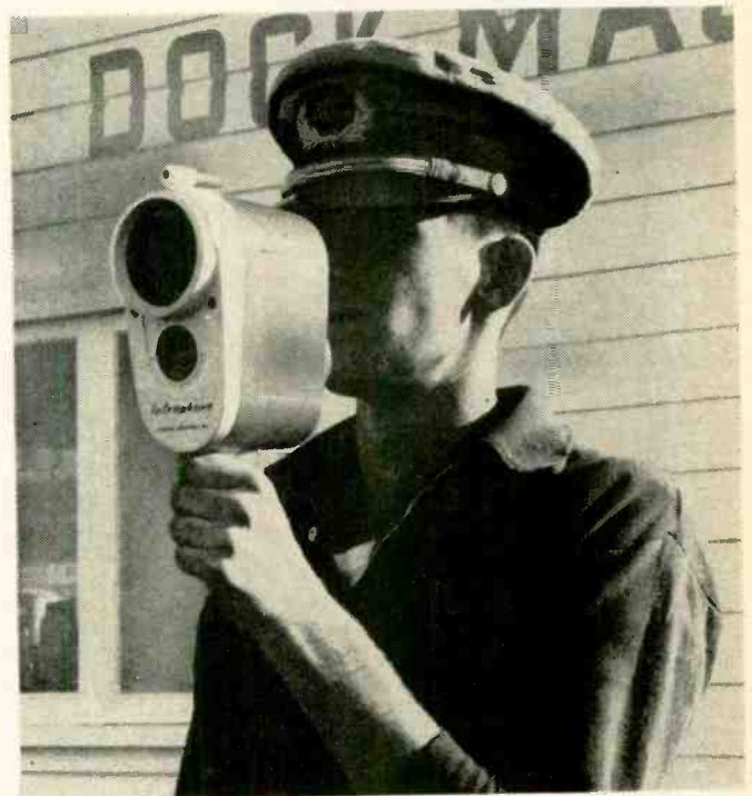
The Infraphone. Large upper circle is receiver detector, smaller lower one, the infrared source.
