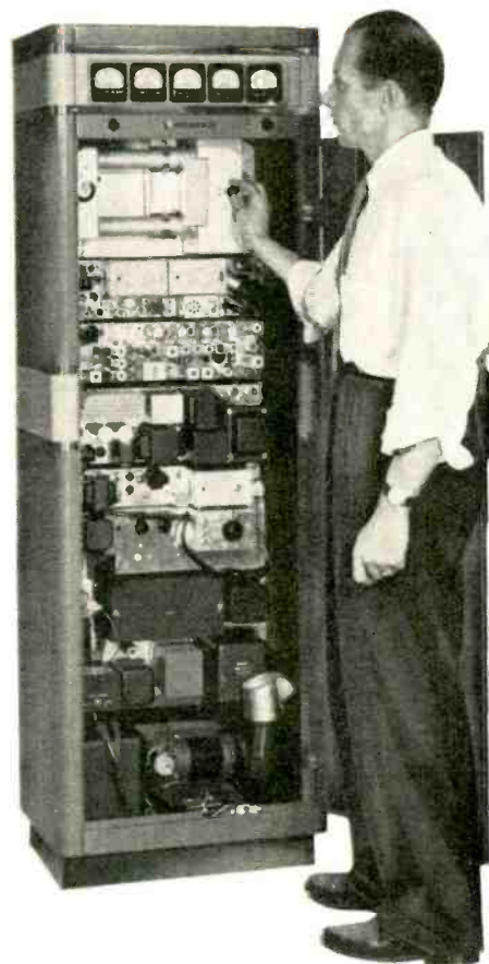
Base station with 250-watt transmitter, made by Motorola, is designed for 450-470-mc operation.
