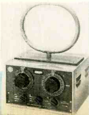
Loop turning control, bearing scale are on front panel of Kaar R238.
