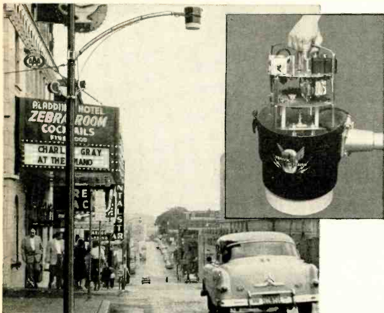
Overhead radar units make a vehicle count for the automatic adjustment of traffic signals. Closeup of radar unit partially removed from its case is seen in inset.
