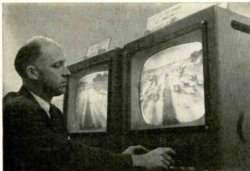
Traffic engineer observes sections of two Detroit expressways via closed-circuit TV during recent tests.
