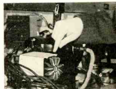
New unit installed on motor has cooling fins, is little bigger than older coil.
