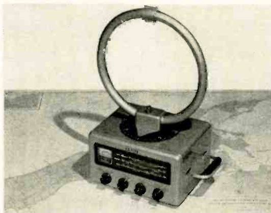
(Above) Roco Radio's RDF has ferrite loop fastened to its case. The entire set is rotated to find null.
