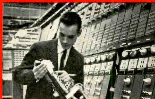
Checking panel wiring of Simpex console
