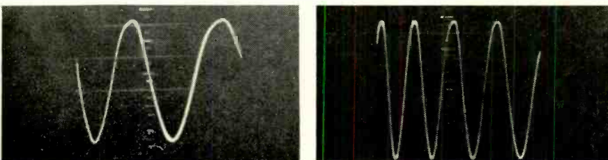
Fig. 2—Oscillograms of the sine wave turned out by the oscillator: a—4 cycles; b—20 cycles.
