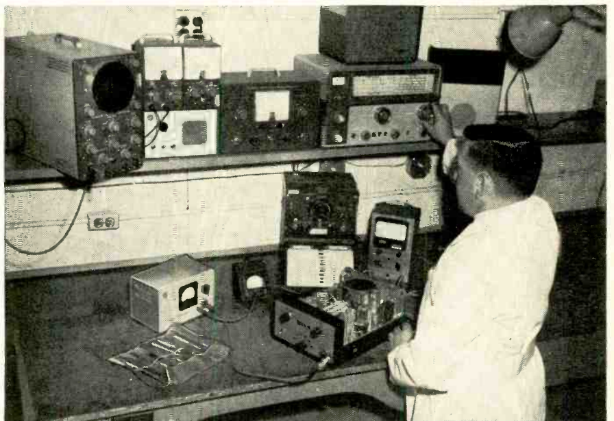
Marine radio channels can be monitored and spurious radiation from a transmitter being checked can be noted with a professional communications receiver.
