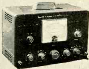
HARMONIC DISTORTION METER
