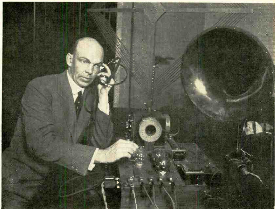
Major Armstrong and his superregenerator, with its 1200- and 1500-turn honeycomb coils.
