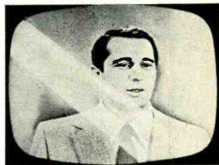
Fig. 5—One complete frame plus part of one field. Taken with Leica on Plus X. Shutter set at 1/30, aperture f2. Focal-plane shutter caused slightly brightened diagonal bar.
