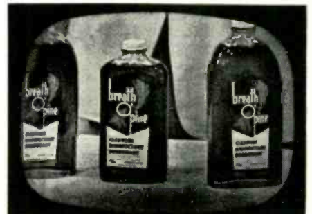
Fig. 2—Normal picture shot at 1/25 with f8 on Rolleiflex. Tri-X film. Correct exposure captures one complete frame.
