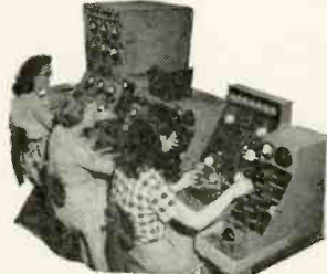
1ST FINISHED TUBE TEST All Raytheon tubes undergo a rigid 100% First Test where they must pass strict requirements on both physical and electrical characteristics. These girls are testing tubes for excessive noise and microphonics, inoperative tubes, specified electrical characteristics and physical appearance.
