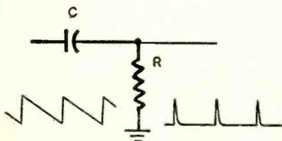
Fig. 11—Simple differentiator network.
