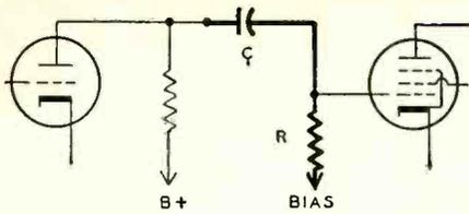
Fig. 6—A resistance-coupled amplifier.
