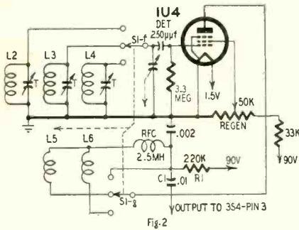
of No. 30 enameled wire closewound at the ground ends of L3 and L4. Adjust the number of turns so the circuit starts to oscillate with 30 to 50 volts on the screen grid. Regeneration is controlled by the sensitivity control.
