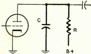
Fig. 10—A basic sawtooth generator.
