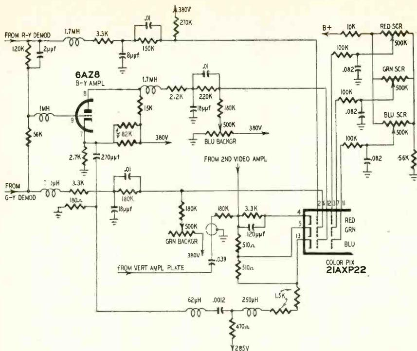
Fig. 3—Diagram of picture-tube element controls in the RCA chassis CTC4.
