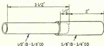
of Plexiglas or Lucite tubing. It is important that the two tubes be overlapped exactly  $\frac{1}{2}$  inch and that General Cement Q Dope, or equivalent, be used to join the tubes together. If desired, the 2-inch section of tubing may be shortened to allow a high-voltage probe to contact the high-voltage measuring point.—*RCA Television Service Tips*
