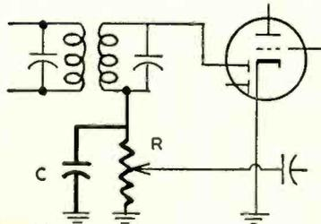
Fig. 7—Basic diode detector circuit.
