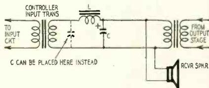
Fig. 5—Adding interference filter.
