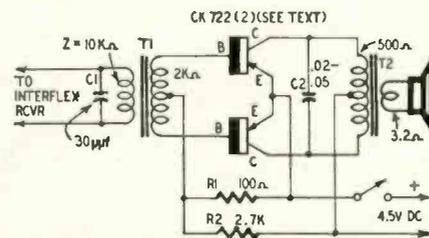
Schematic diagram of the push-pull audio amplifier for the Interflex tuner.
