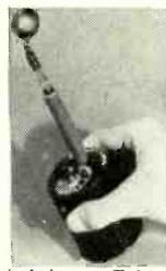
With the attachable pick-up loop, (where sufficient signal is available) the Probe Meter can detect and indicate radiation of signal thru I.F. and video amp tubes. (Simply slide loop over tube being tested.) Where internally shielded tubes are encountered, remove tube and insert probe tip into grid pin of socket. Indicates gain per stage.
