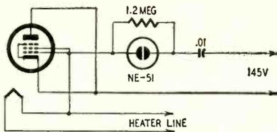
Fig. 3—Circuit for testing pentodes.
