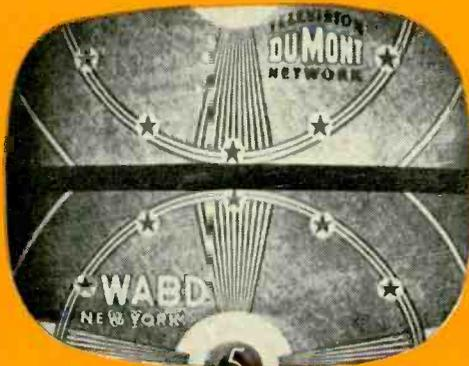
Fig. 1—Appearance of blanking signal.
