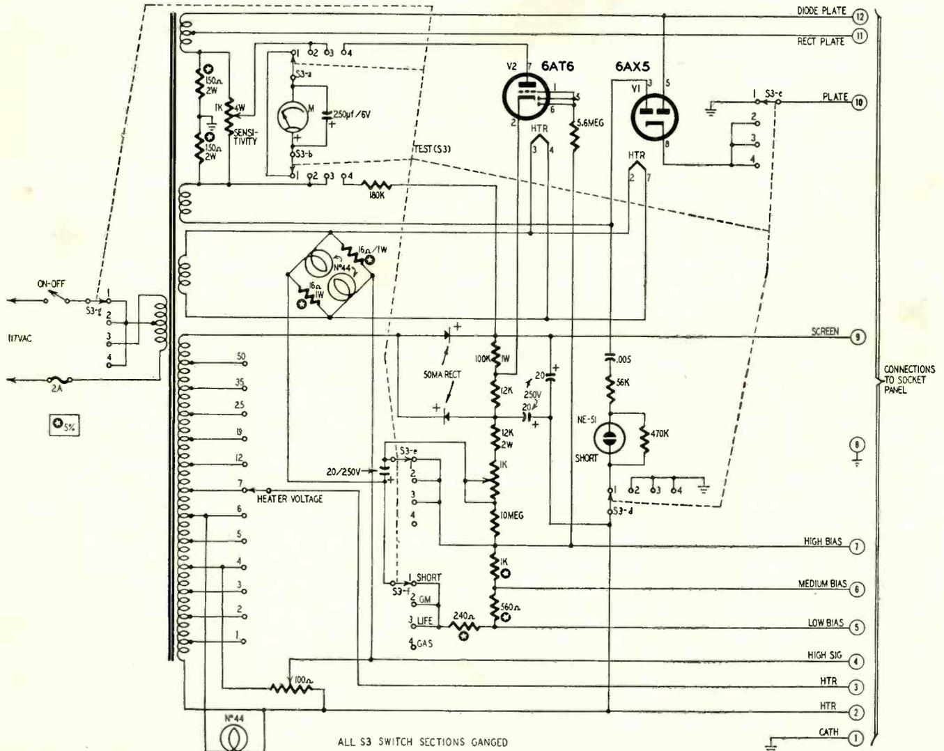
Fig. 4—Simplified schematic diagram of the model 500 Dyna-Quik tube tester.
