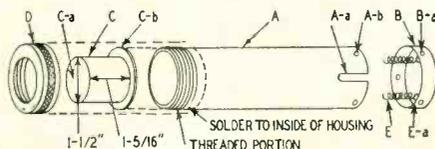
**Fig. 1—Probe assembly for phototube.**
