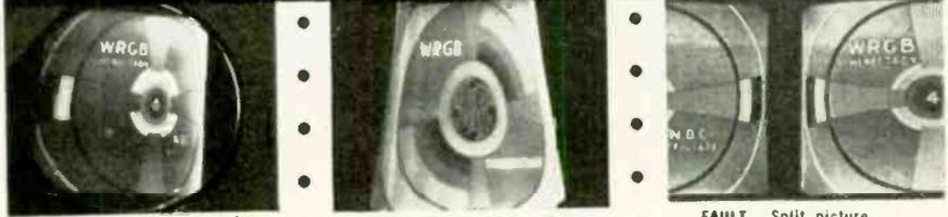
**FAULT**—Picture compression and stretching.
