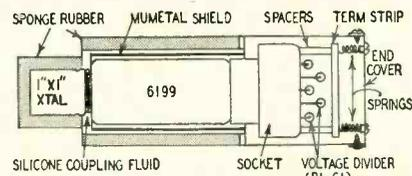
**Fig. 2—Cross-sectional view of probe.**
