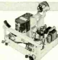
Advanced Cascade turret • AFC horizontal sync. • 3-stage sync. amplifier, clipper and separator • 4-stage stagger-tuned video IF • Adjacent-channel trap • 2-stage video amplifier • Direct-coupled keyed AGC circuit • 5 microvolt sensitivity • For 21" to 27" (90°) picture tube.
