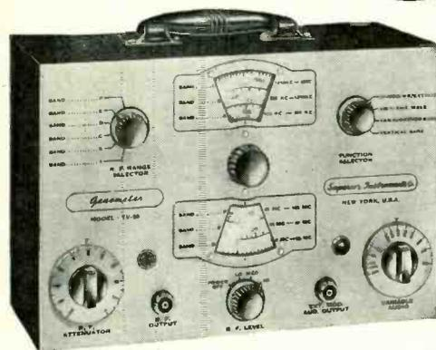
**CROSS HATCH GENERATOR:** The Model TV-50 Genometer will project a cross-hatch pattern on any TV picture tube. The pattern will consist of non-shifting horizontal and vertical lines interlaced to provide a stable cross-hatch effect.
