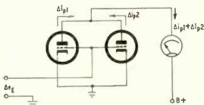
Fig. 5—Measuring g<sub>m</sub> of dual tubes.
