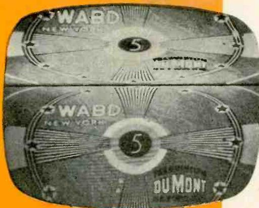
Fig. 4—Vertical frequency at 30 cycles.
