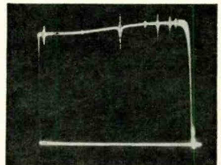
Fig. 3—Video sweep response. A 4.5-mc marker in center of pattern—spurious markers are above and below this point.
