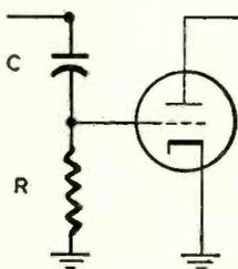
Fig. 9—Circuit for grid-leak biasing.
