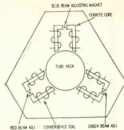
Fig. 4—A typical convergence yoke.
