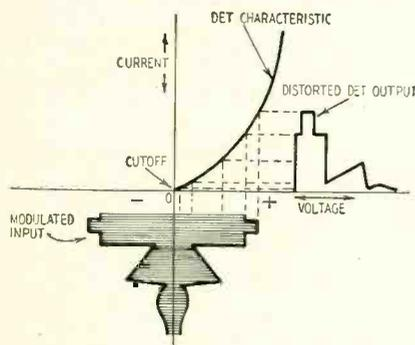
Fig. 1—Crystal detector characteristic.
