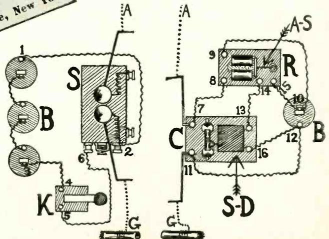
Mounted on the spark coil, on two metal standards, were two brass oscillator balls between which a small blue spark jumped the 1/8-inch gap. The spark coil had a fast vibrator so that every time you depressed the key a spark would jump between the two balls. Depressing the key for a short period would give a dot, a longer period would give a dash.
