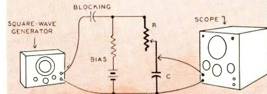
Fig. 1—Setup for time-constant study.
