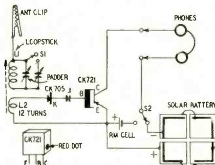
Fig. 1—Schematic of the receiver.
