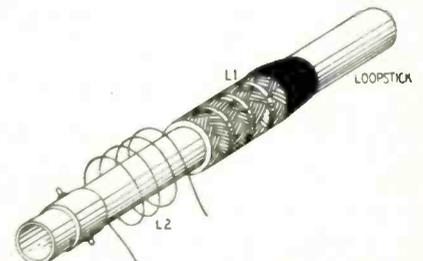
Fig. 2—Windings on the loopstick.
