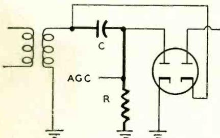
Fig. 8—Diode circuit for agc takeoff.
