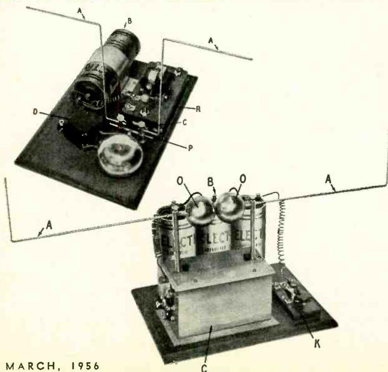
Replicas of the original transmitter and receiver, soon being sent to the Ford Museum at Dearborn. Left—the receiver: A, antenna system; B, dry cell; C, coherer; D, decoherer; P, adjustable coherer rods; R, 75-ohm relay. Right—the transmitter: A, antenna and counterpoise; B, dry-cell power supply; C, 1-inch spark coil; O, spark-ball oscillators; K, transmitter key.
