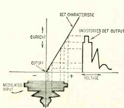
Fig. 2—Undistorted detector output.
