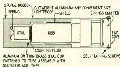
**Fig. 3—Diagram of a simplified probe.**
