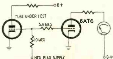
Fig. 6—Grid emission test circuit.
