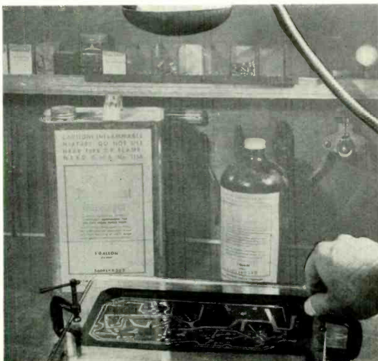
Equipment and setup for exposing the sensitized laminate.
