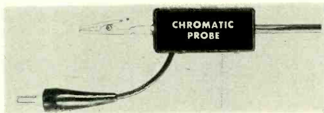
Below — the Simpson chromatic probe—has crystal rectifier.
