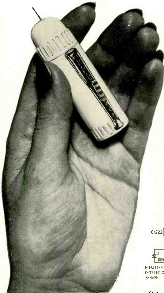
The completed signal injector.
