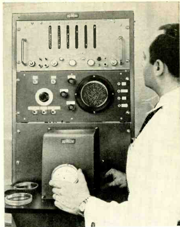
Du Mont's Iconumerator , a device which can count objects of any size and shape in its field of vision. Here its subjects are similar to colonies of bacteria counted in medical laboratories, etc. The most startling feature of the instrument is that the size of the object (as long as it can be contained in the field) or its shape make no difference in the accuracy of the numeration.
