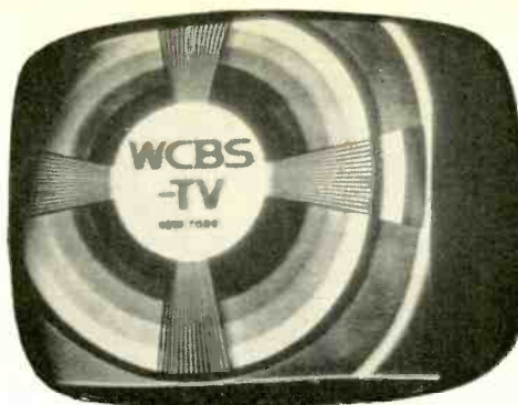
Fig. 2—Video amplifier overpeaking.
