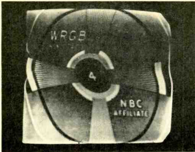
Fig. 2—Sixty-cycle hum modulation.
