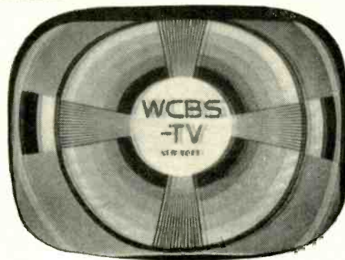
Fig. 2—Video amplifier overpeaking.
