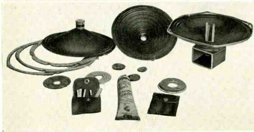
All the equipment needed to replace cones—plus two finished jobs—appears above.
