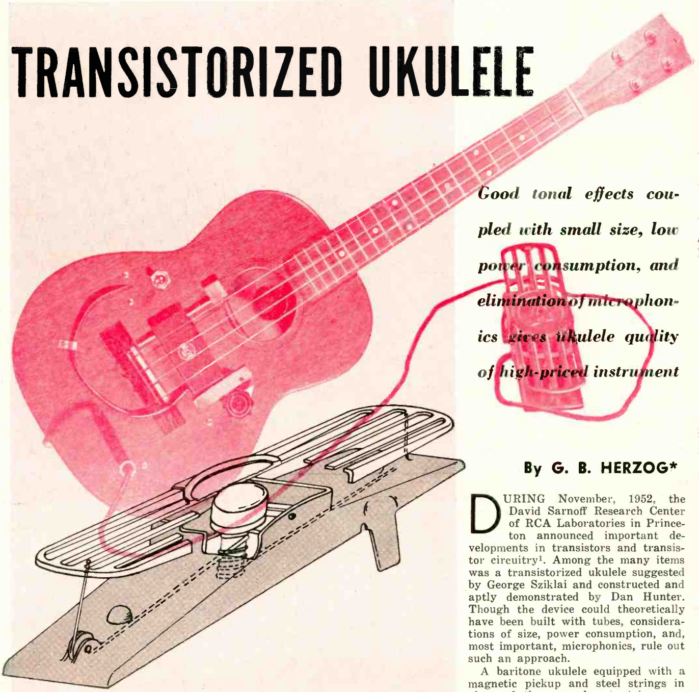
Foot movements vary potentiometer to provide convenient volume control.
