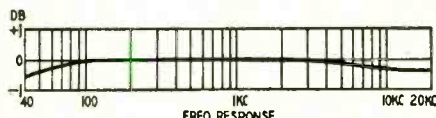
MEASURED ON HEWLETT-PACKARD 200AR OSC & G-E VU PANEL WITH DAVEN MEASURING SET
