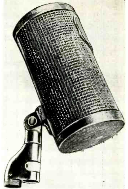
Fig. 3—The finished microphone housed in an air-freshener can. All-around perforations are essential to allow free passage of air through the microphone.
