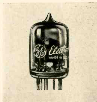
G-E 6AJ4 grounded-grid u.h.f. triode.
