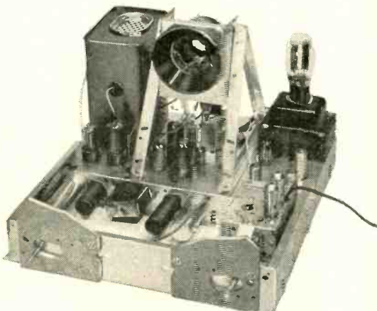
The above-chassis views of two Sonoras show improvement in heat radiation. Capacitors are mounted in cool area.
