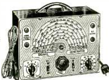
* Tubes used: One 554 as oscillator; one 954 as modulated buffer amplifier; T-2 as modulator; 7193 as rectifier.
