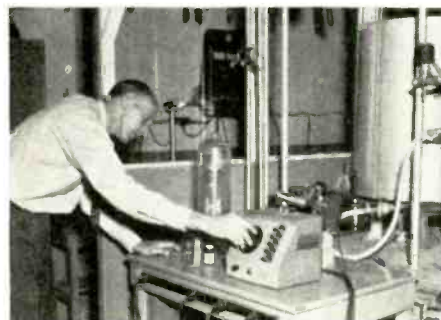
Careful study of the formation of thin metallic films in a vacuum . . . basis for the aluminizing of tubes.
