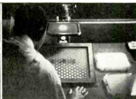
Inspection and checking of perforations .0075" in diameter in masks of tri-color picture tubes.
