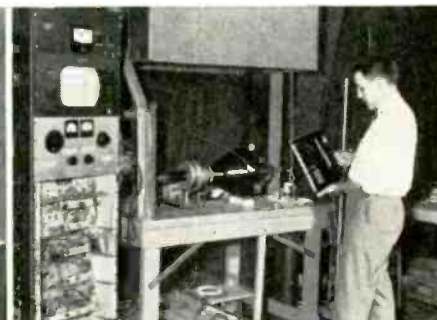
A physicist using a Rauland-developed radiation meter in checking X-ray radiations from cathode ray apparatus.
