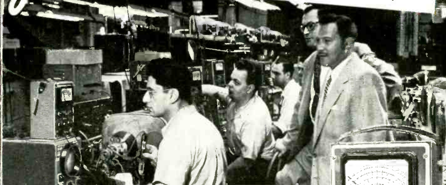
Mr. Al Goldberg, Assistant Chief Engineer of CBS-Columbia and Harry R. Ashley, President of EICO, inspecting the use of the EICO Model 221 Vacuum Tube Voltmeter and Model HVP-1 High Voltage Probe at the Sweep Frequency Troubleshooting Position on the CBS-Columbia Television production lines.
