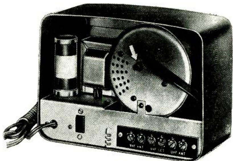
Fig. 3—Rear of Kingston converter. Large cylinder is the tuner.
