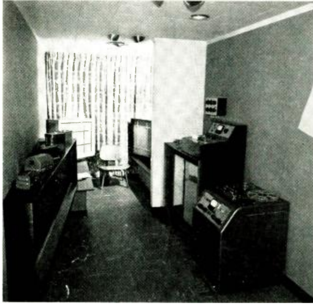
Part of the trailer interior. Mixer console and tape reproducer are at the left. Special acoustic treatment was needed to overcome space limitations.
