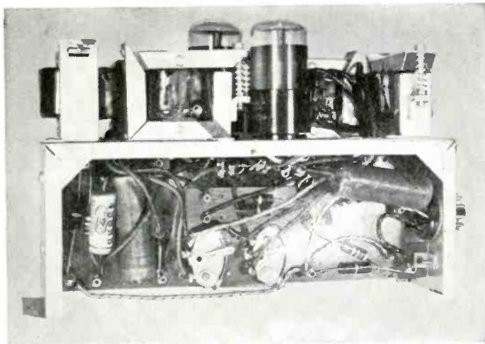
Fig. 4, left—This oscillator chassis generates four tones in the Model 2A2. Fig. 5, right—Rear view of a Connsonata shows how oscillators, power supply, boosters, preamplifier, coupler relays, and power amplifier are mounted inside the console.
