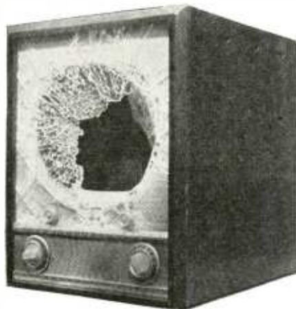
Front view of set damaged by implosion.
